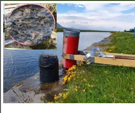
Figure 3. Core sampler with inset of 15 cm cross section.
