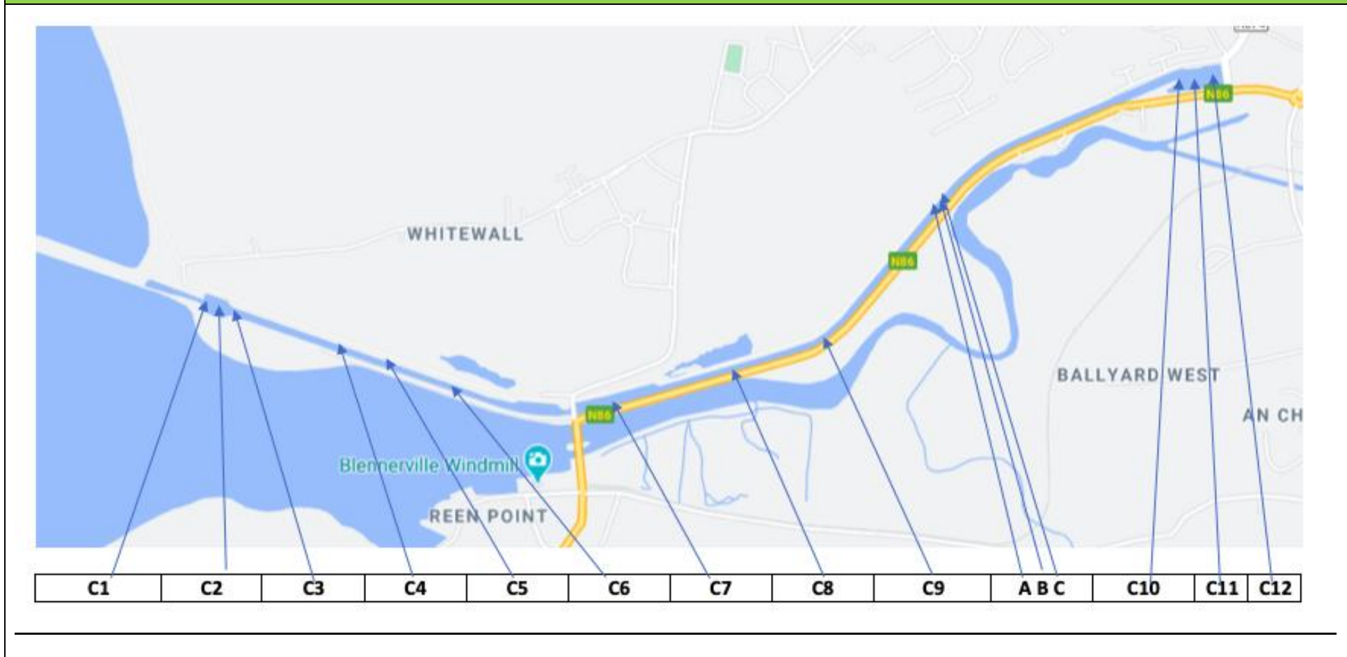
Figure 4. Location of samples from centre line of canal (C1-12) and from pocket of sediment in damaged N wall close to surface (A,B,C)
